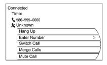
**Switch Call:** Turn or press the MENU/SELECT control knob to "Switch Call" and press Enter or press the "Switch Call" option.
